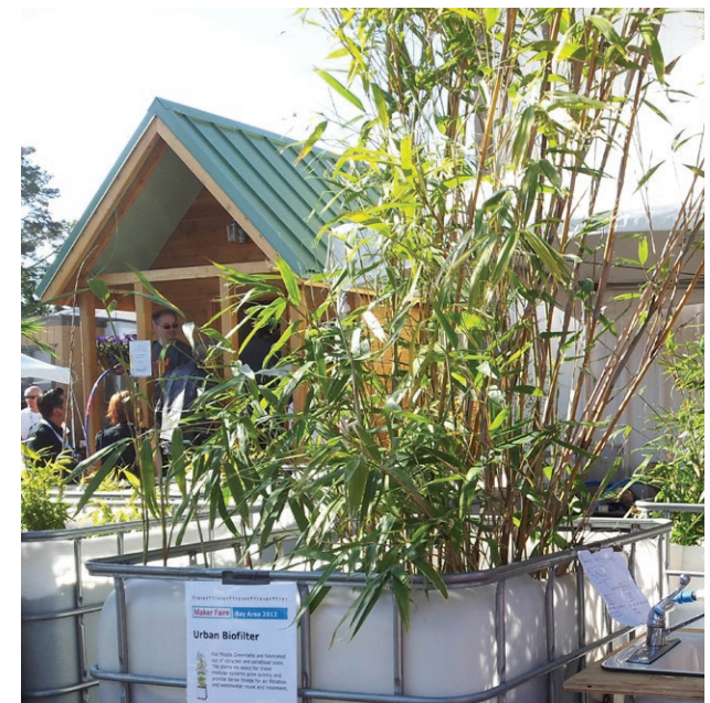
Small scale greywater treatment with bamboo filter. Credit: urbanbiofilter.org
